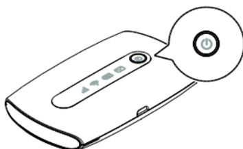
Press and hold the
